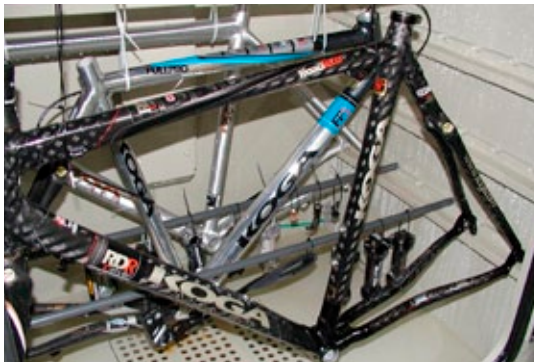
Salt spray test
