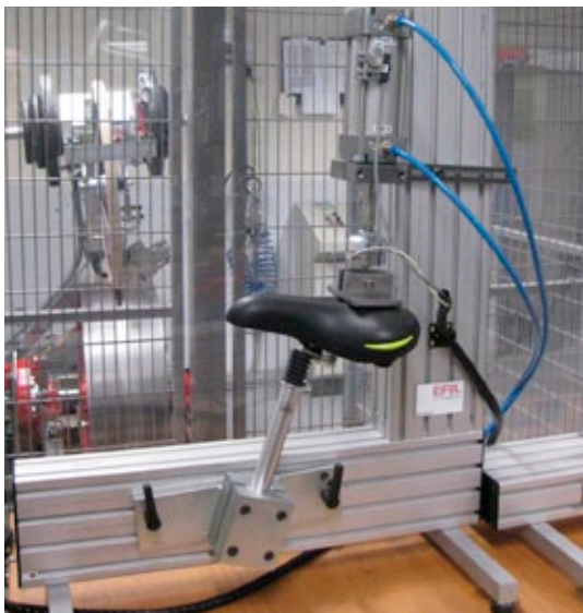
Saddle pin test
